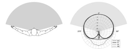
Figure 3a. Typical pick-up area (with full frequency response) of an Earthworks cardioid microphone indicated by extending arms
