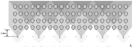
Figure 8 below, shows that it would actually take 12 conventional cardioid microphones to provide the same coverage as 3 Earthworks cardioid microphones, when placed 3 feet in front of the choir.
