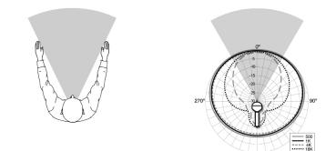
Figure 2a. Typical pick up area (with full frequency response) of a conventional cardioid microphone indicated by extending arms
