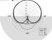
Figure 10. Rear Polar Response of an Earthworks Cardioid Microphone
