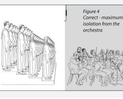
When miking choirs with an orchestra or band in front of the choir, the microphone head should be perpendicular to the floor to provide the greatest amount of isolation from the orchestra or band.
