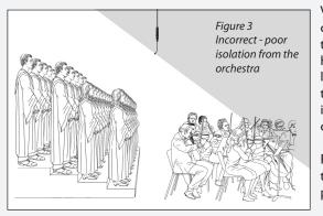
When miking choirs with an orchestra or band in front of the choir, the microphone head should be perpendicular to the floor to provide the greatest amount of isolation from the orchestra or band.
