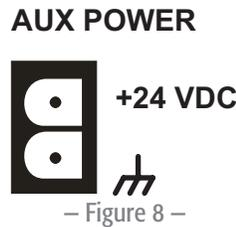
**CAUTION!** The power supply used to provide 24 VDC power to the unit shall be a UL Listed ITE power supply, marked LPS, or a UL Listed direct plug-in power unit, marked Class 2, with a rated output of 24 VDC/500 mA.
